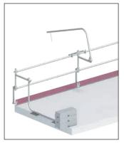
In the case of a flat roof without fascia, both flat roof guardrail posts (Ref. Nos. 2666.010 and 2666.011) are used. It must however be ensured that the 3-piece side protection (handrail, knee rail and toe board) is provided without fail. With the flat roof toe board holder, the guardrail posts (slide preventers) can be supplemented by Speedy toe boards if there is no roof upstand.
